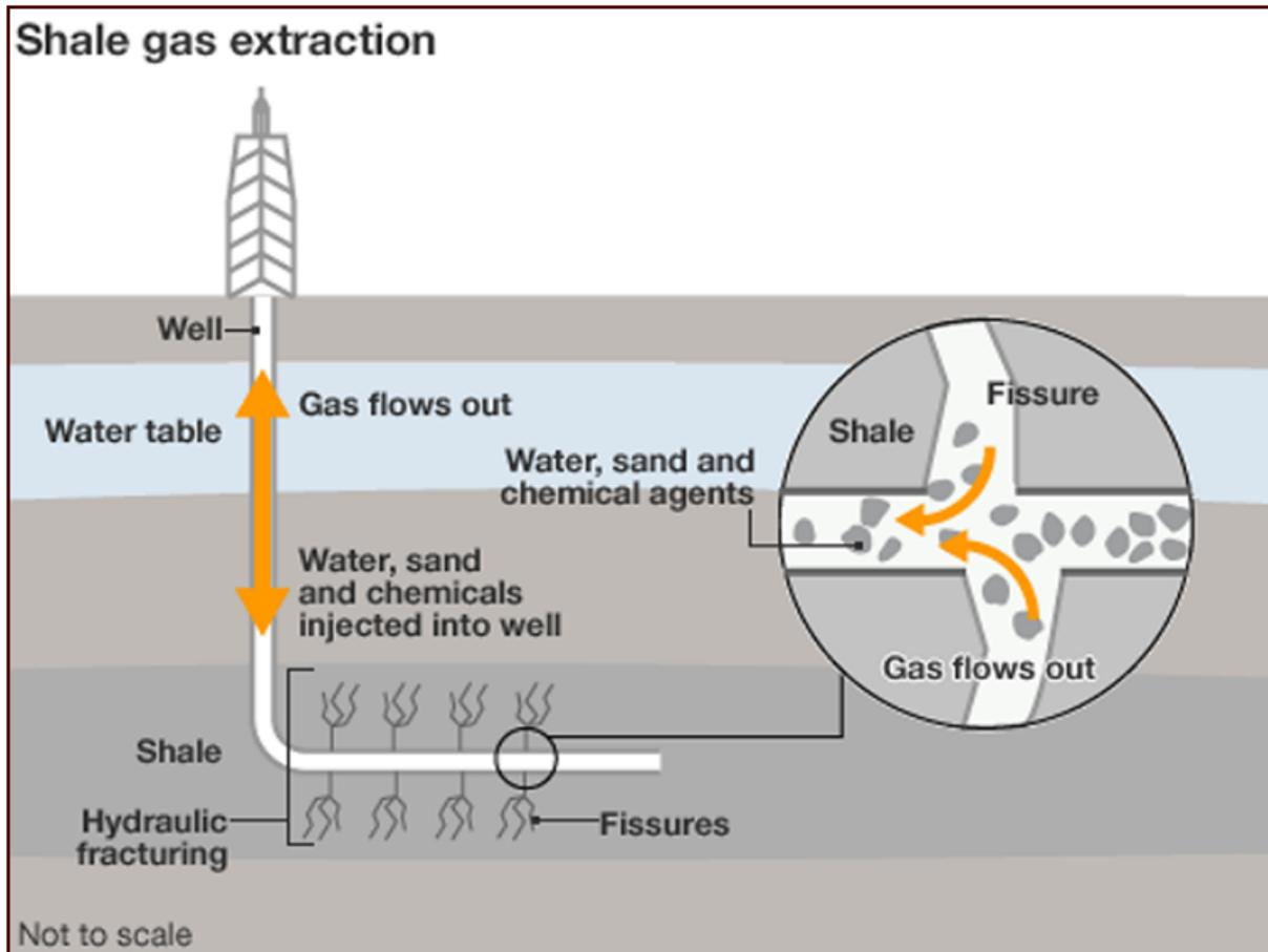
**Figure 2-1 Principles of shale gas extraction**
