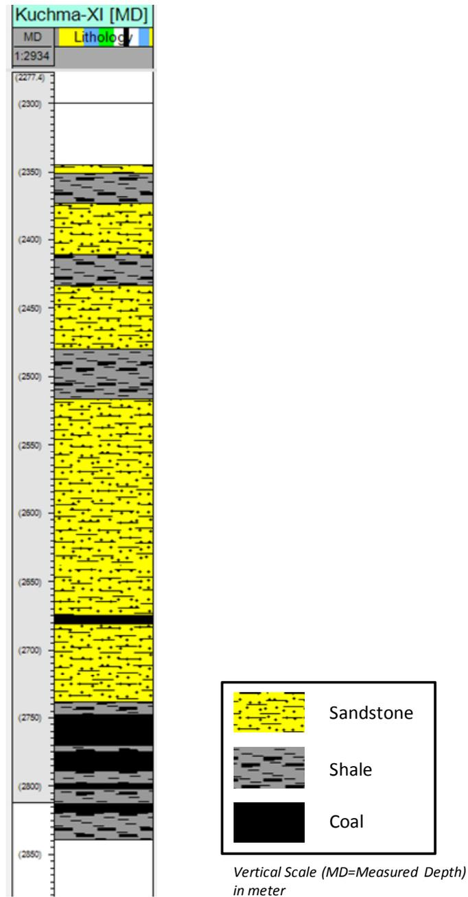
**Figure 4-6 Simplified Lithology of the Kuchma Formation in borehole Kuchma-IX**
