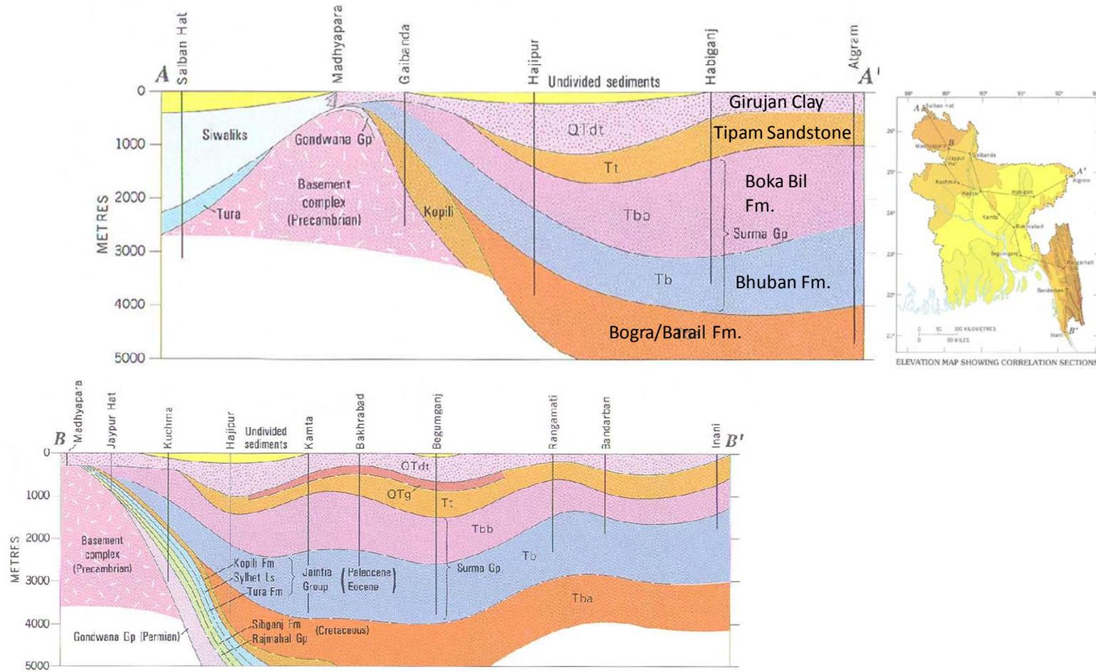
**Figure 4-4** Structural cross-sections across the Bengal Basin showing the sedimentary cover
